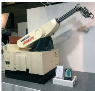
Fig. 6. Primul robot industrial programabil Unimate
